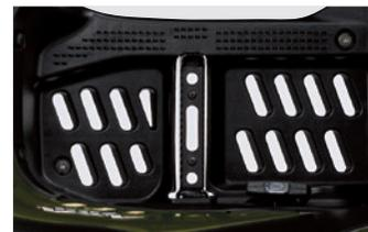
Full floorboards with drain holes
